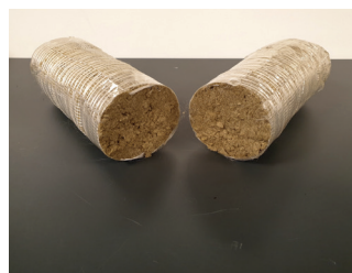
Cordon coupé correctement / Properly cut rope.
