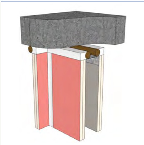
FS703 plasterboard to concrete linear gap seal with PE backer rod: EI120
